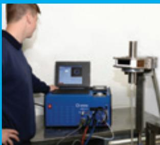
nents our orbital welders can provide the "perfect weld" for customers that require continuity, quality and a high level of consistency. By using detailed welding procedures which are stored in the machine's memory and quickly retrieved, our tubular components can be rapidly reproduced to the same specification providing comprehensive weld data logging for customers requiring full traceability.
