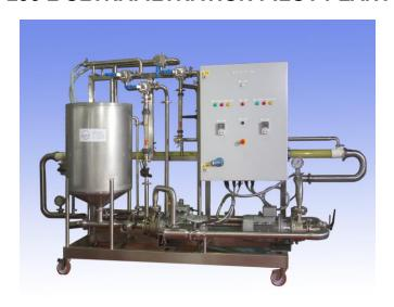
Designed for pilot scale Microfiltration and Ultrafiltration trials
